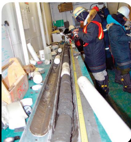
Researchers at the Mallik site in northwestern Canada retrieve drilling cores containing methane hydrates.
